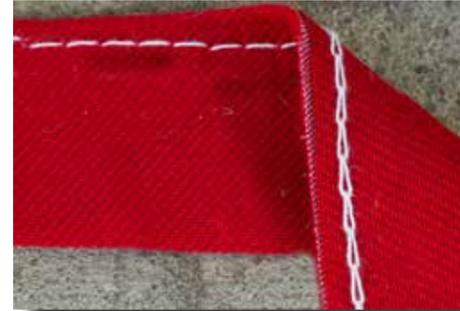
The machines produce single thread chain stitch seams. For increased tear resistance there is the option "two needle execution". Then, the machine produces two parallel seams. For 621/622 the distance between the two seams is 6mm whereas for the 721/722 the distance is 10mm.
