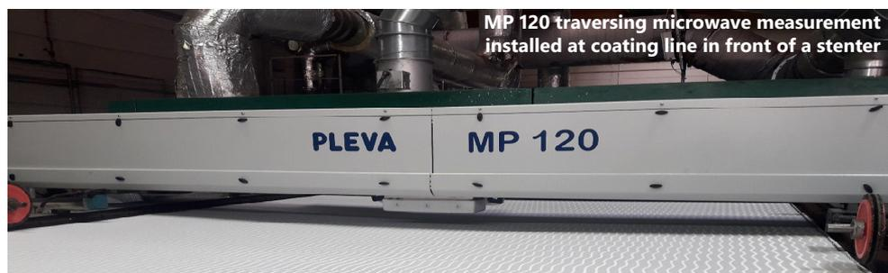
MP 120 traversing microwave measurement installed at coating line in front of a stenter
