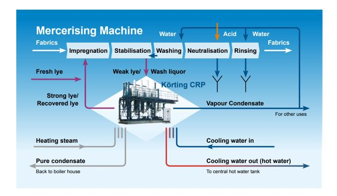
The vapour condensate is slightly alkaline soft water without any hardness. It has a temperature of approx. 90°C. It can be
