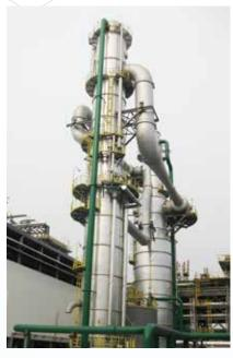
Bridge design, self-supporting (without separate steel construction), 2-tower design, 3-stage, countercurrent plant
