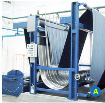
A. Entrance frame for feeding denim in rolls arriving from looms or on A-frames
