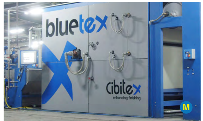
M. Felt calender diameter 2.500 mm
