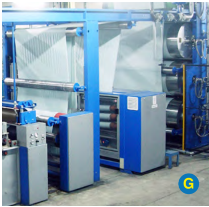
G. High tension unit for stretching and weft-straightening process to prevent the twisting of denim
