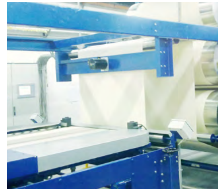
Pick counting system for the control of fabric shrinkage
