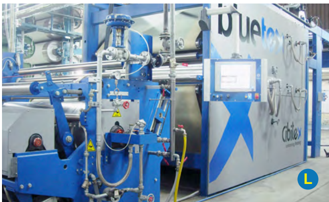
L. Compressive rubber belt shrinkage unit
