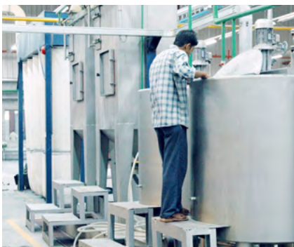
Wet and dry cleaning filters to collect dusts and release clean air
