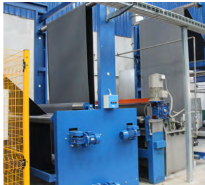
Triple rollers fabric skewing unit with high tension stretcher
