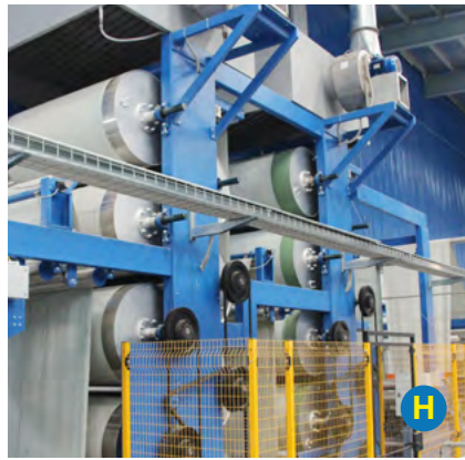
H. Can dryer with rollers diameter 800 mm
