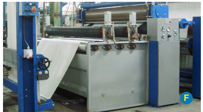
F. Wet finishing process for the application of finishing liquor in an uniform and deep application
