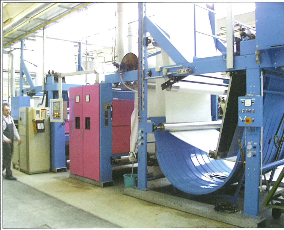
配有 J 型箱的烧毛机生产线 Singeing range with J box.
