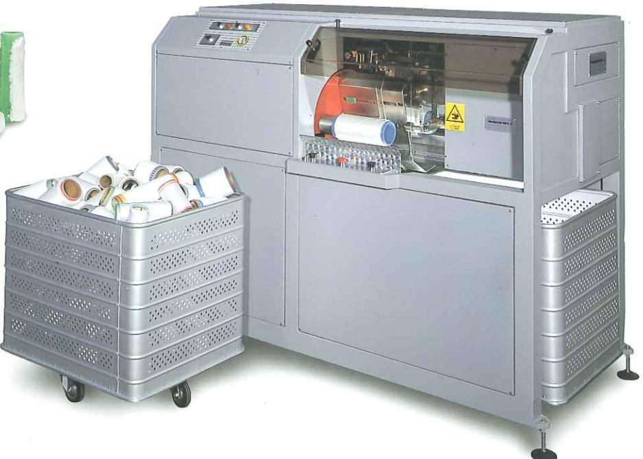
*The full automatic yarn-cutting group, expressly developed to save and reuse the tubes, assures safe operations.*
