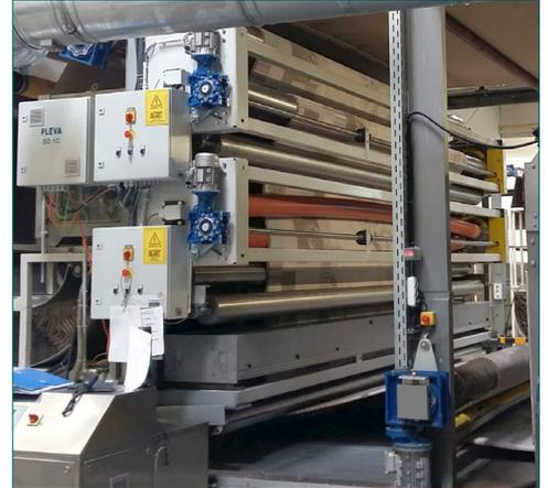
SL C: Modular straightening system for carpets
