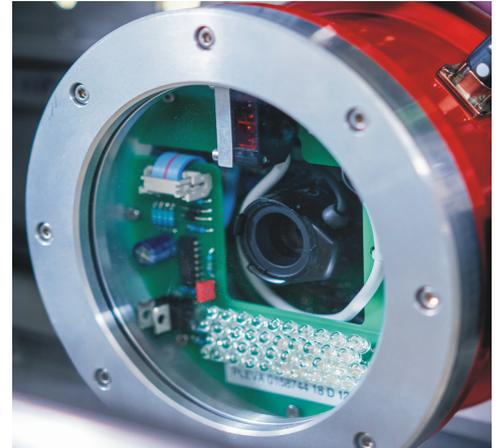
CAM series 300: fabric sensor, lens and LED front flash
