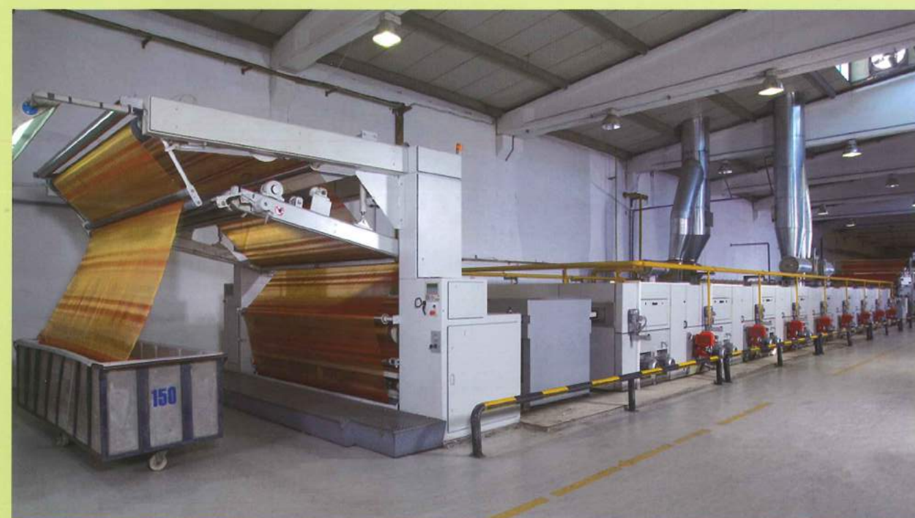
Stenter with horizontal chain system and gas heating
