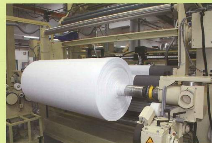
Movable batcher on a mobile platform for the batching of delicate woven and knitted fabric
