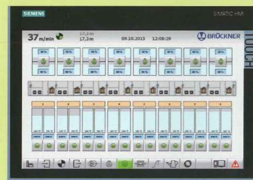
Details of the dryer with temperature profile as bar chart
