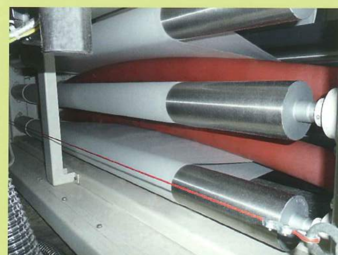
View into the integrated weft straightener in the stenter entry
